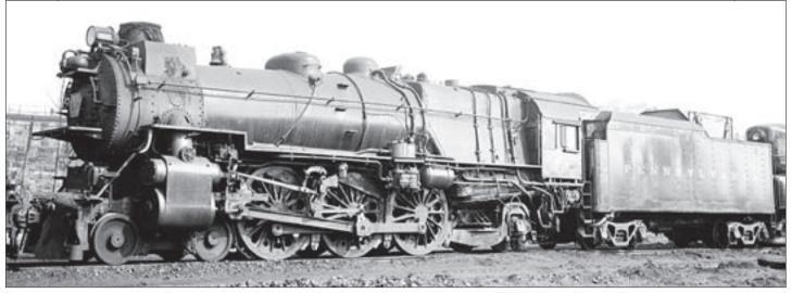
Shown above is #612, a K-4sa version with 130P75 tender equipped with radio equipment. The most distinguishing feature of the 'sa' is the front-end throttle box mounted on the smokebox. The 'sa' also had larger cylinders and they were the 'hot rods' of the K-4 class. (post 1952 service period)
