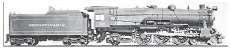
Above is an 'As Built' 5400 series K-4 in full passenger dress, which includes striping on the cab, tender and wheel-sets. The tender is a 110P70 without stoker (1927-30 service period). The 'Early' version is the same as the previous configuration minus the striping (1930-36)
